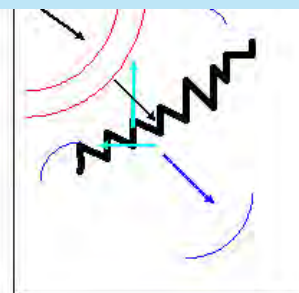
Diagram 1-15. Effect of diffuser-element boundary on sound wave.
